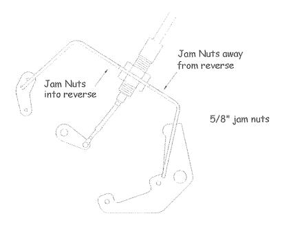
Small adjustments (1/6 of a turn) made with both jam nuts makes a noticeable difference. A smooth shift sequence is therefore attainable first through fourth gears and reverse.
