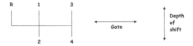
Push the shift rod coupler into first gear and loosen the two 5/8" jam nuts on the gate cable. Gently slap the shift handle up against the Cable-Shift lock out bar. Screw the 5/8" gate cable jam nuts towards one another and finger tighten against either side of the gate cable bracket. The Cable-Shift shifter should be close enough to 'run through the gears'. Shifting will improve when the engine is running and the clutch is depressed. Shifting further improves as the synchronizers are worn in.
